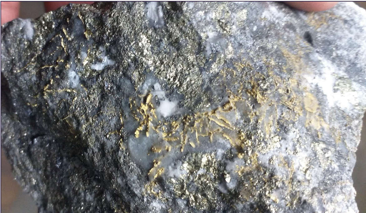
Figure 1. Hand sample of high-grade Au in polymetallic vein mineralization from the Tangana 1 vein, level 650 (4650 masl).
